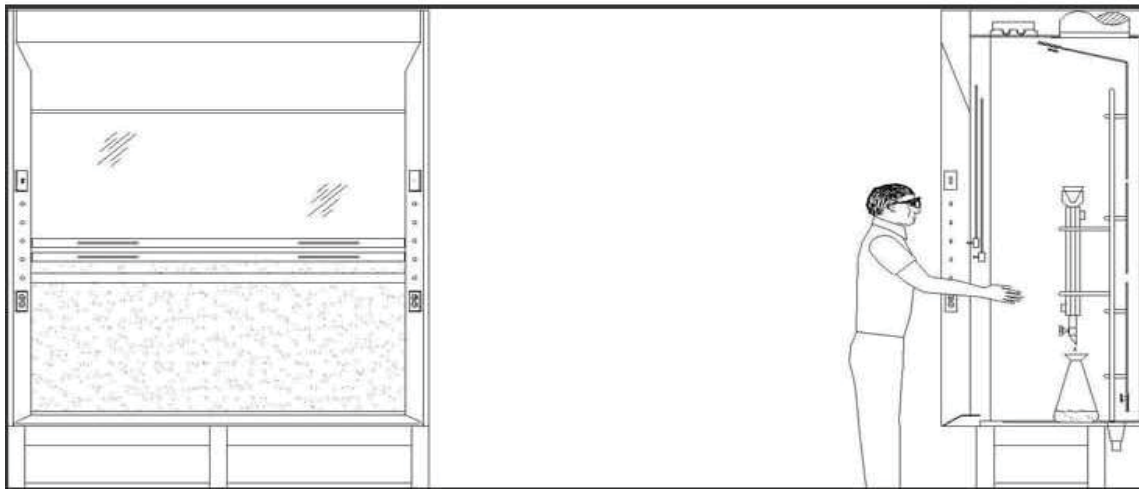
Fig. 7 Typical View of Distillation Fume Hood
